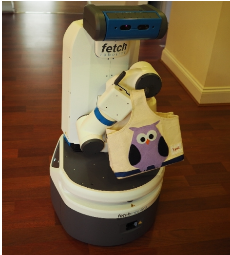
Fig. 1. The Fetch robot at Robot House, its arm configuration, and the basket used for the experiment.
