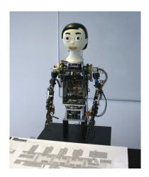
Fig. 1. Picture of the hardware setup. The robot torso BARTHOC with the Flobi head has been placed behind a desk to act as a receptionist.
